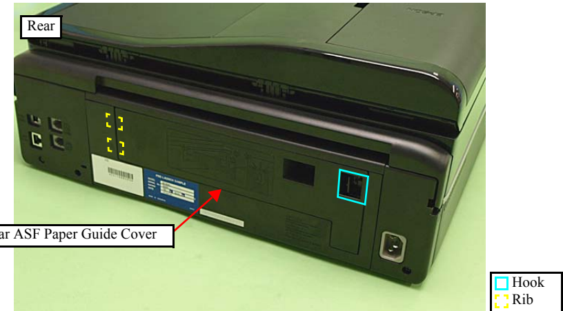
Figure 4-25. Removing the Rear ASF Paper Guide Cover
