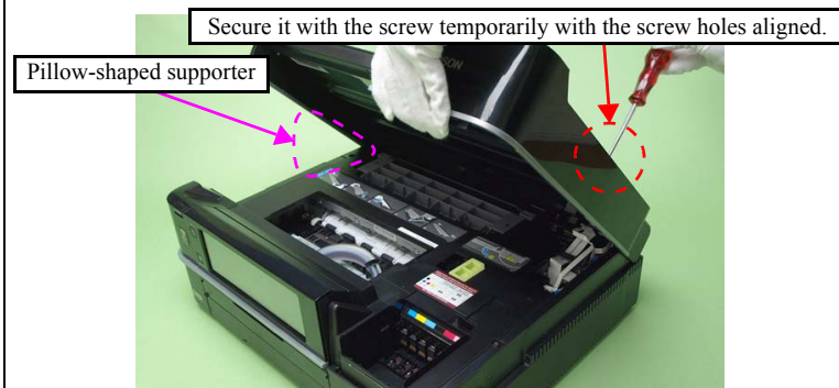
Figure 4-10. Installing the Scanner Unit (2)
