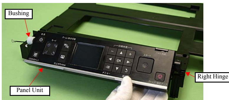
Figure 4-228. Removing the Panel Unit (3)
