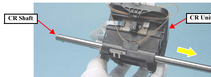
Figure 4-91. Removing the CR Unit (4)
