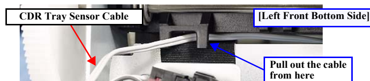
Figure 4-111. Routing the CDR Tray Sensor Cable
