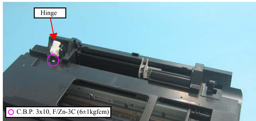
Figure 4-10. Removing the Hinge
