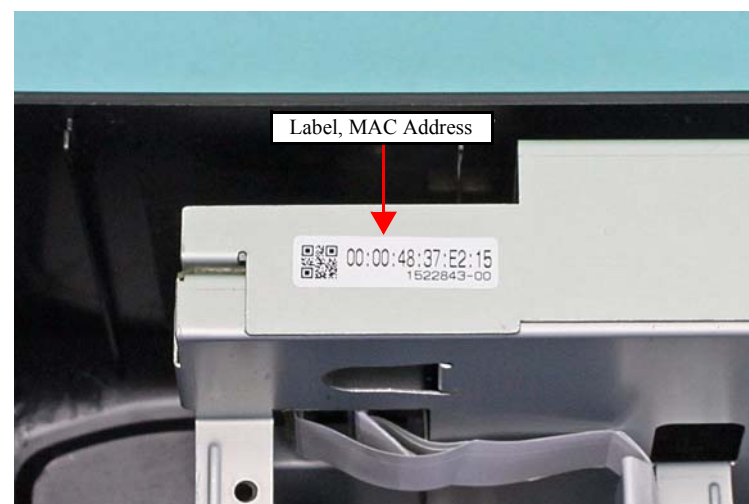
Figure 7-44. Position to attach the MAC Address Label
