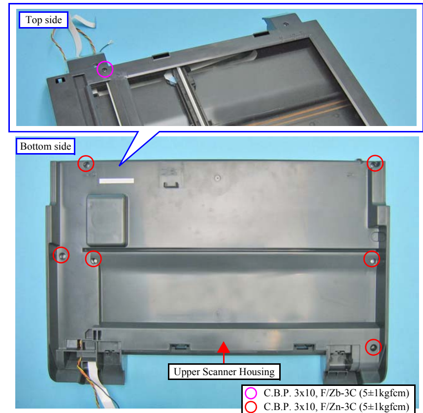
Figure 4-102. Removing the Upper Scanner Housing (1)
