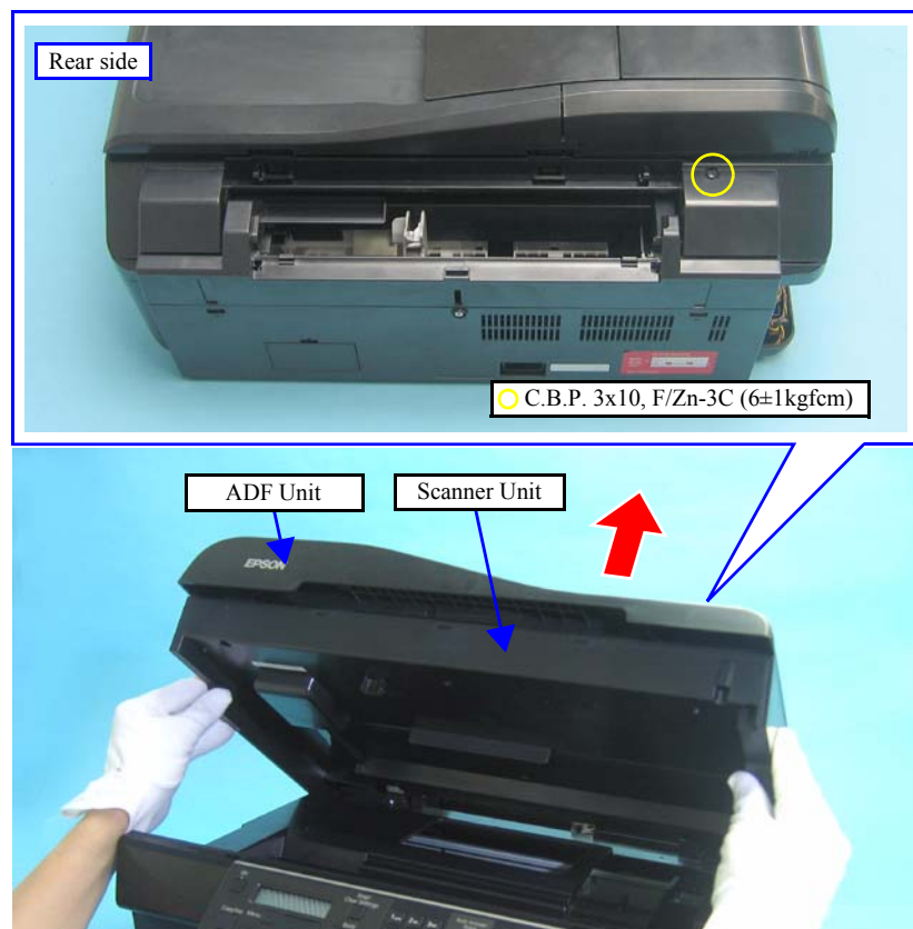
Figure 4-6. Removing the Scanner Unit/ADF Unit (2)
