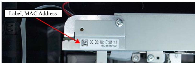
Figure 7-13. Position to attach the MAC Address Label
