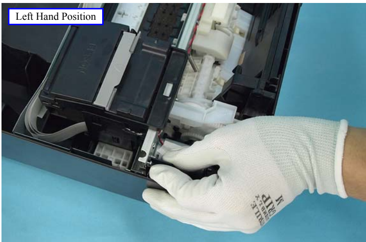
Figure 4-42. Printer Mechanism Handling Precaution
