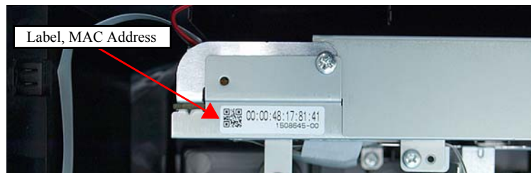
Figure 4-23. Position to attach the MAC Address Label
