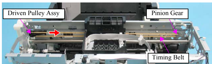
Figure 4-131. Removing the CR Motor (2)
