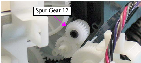
Figure 4-163. Handling the Spur Gear 12
